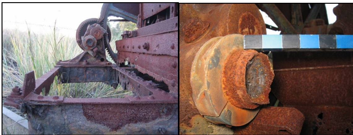
Figure 8.1: Signatures of salvage on Steam Crane Barge 3. (Left) An empty engine mount and (Right) evidence of cutting on the crankshaft (Images by author).
