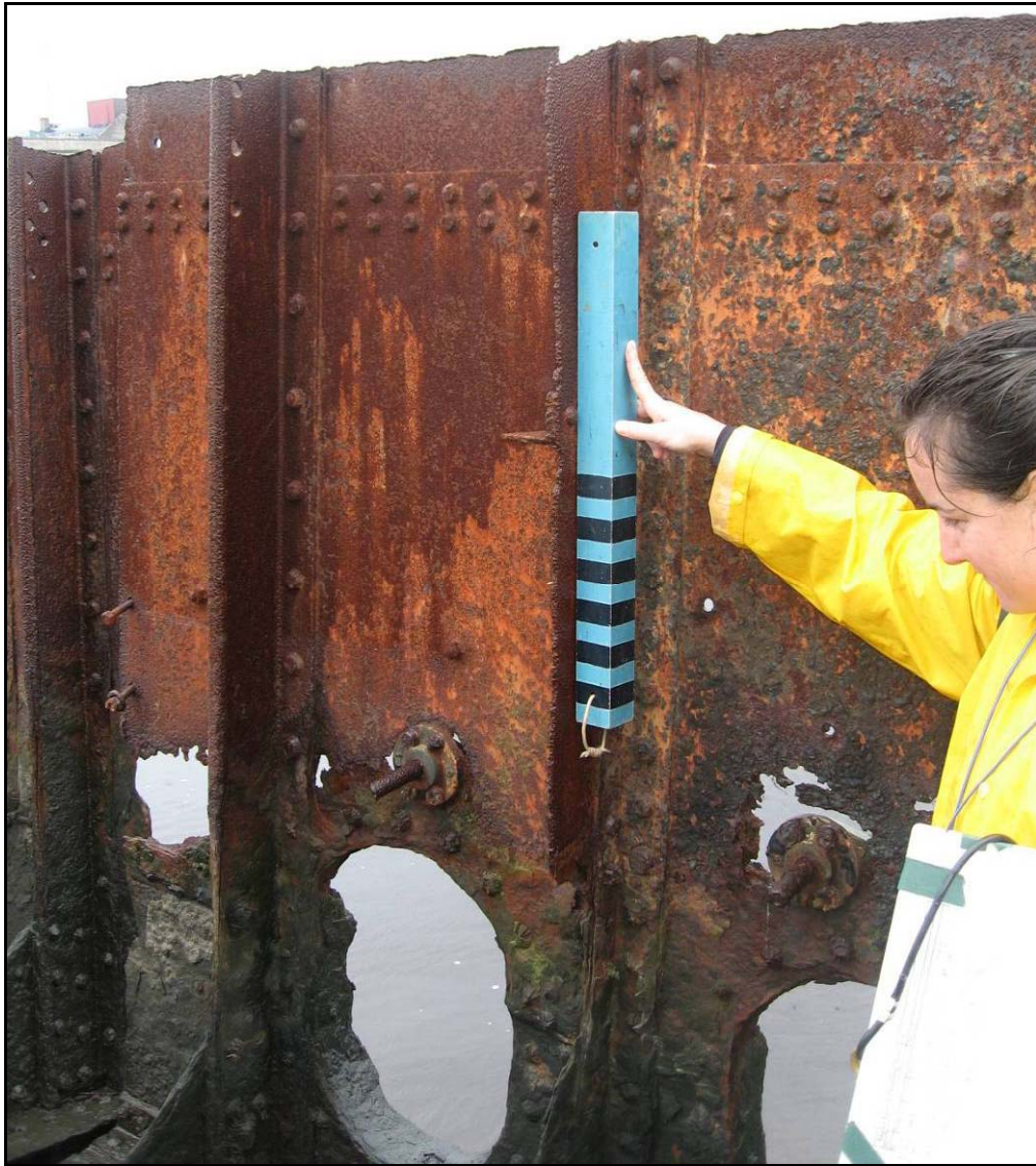
Figure 8.3: Evidence of cutting on a bulkhead and at the top of the structure of Stockpile 1/ Stone 20 (Image by Nathan Richards).
