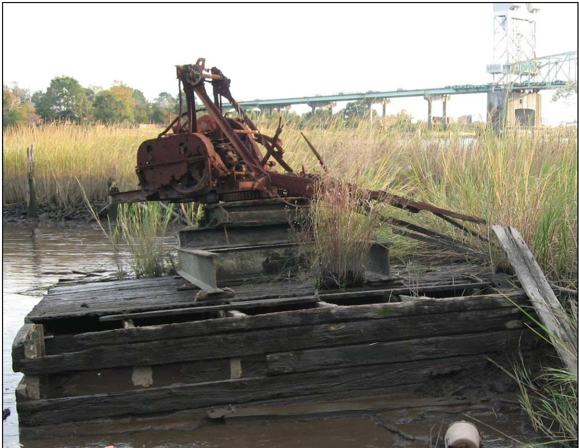
Figure 6.17: Steam Crane Barge 3 with intact derrick machinery (Image by Tiffany Pecoraro).
