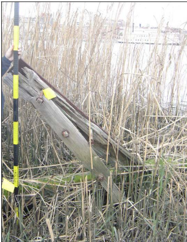
Figure 7.5: Remains of A-frame in situ on the snag boat H.G. Wright (Image by Joe Hoyt).
